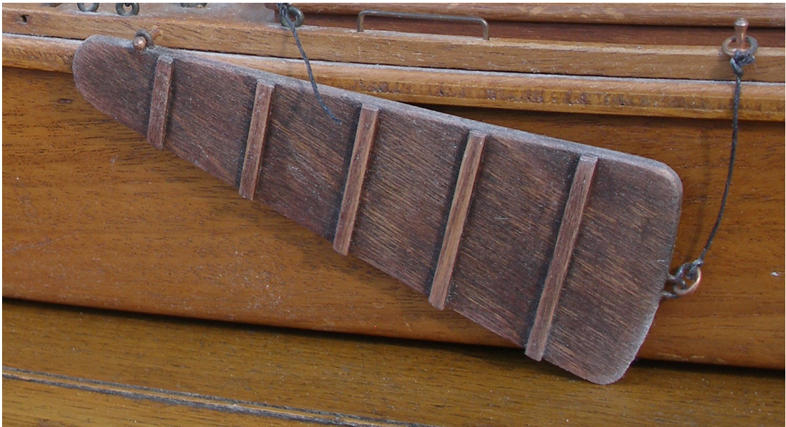
Lee boards were hung either side of the vessel. Either could be lowered to serve as a keel on the lee side – opposite to windward
